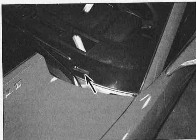
The Vehicle Identification Number (VIN) is visible through the driver's side of the windshield
