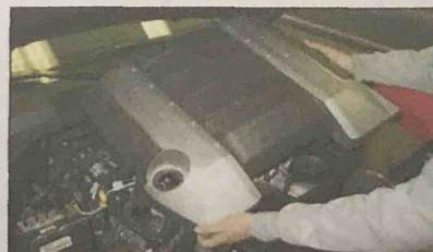
3. Remove the oil filler cap and then lift up and remove the engine cover. Reinstall the oil filler cap.
